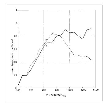
Fig 9 (Source ref 4) Absorption Coefficient of 50 mm glass wool, mounted immediately on concrete a) uncovered, b) covered by a panel of 5mm thickness, perforated at 14%.
